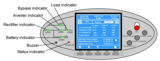
The current operational status of the Liebert<sup>®</sup> NX<sup>™</sup> is indicated by the color of the indicators—green, amber or red—and whether they are ON (solid), flashing or OFF. **Table 27** provides a guide to interpreting the various states of the indicators.
